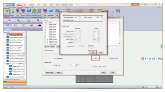
b. Select the input interface(need to change the input resolution) and change the resolution to 1512 \* 1344 , then click application(some PC need to re-plug the signal or restart the computer to take effect).
