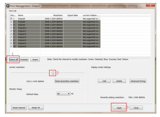
c. Set the output layout, enter the splicing setting and select the resolution as 1512\*1344, select the large screen combination as 1\*8, align the grid line to 2\*16, then select the synchronization mode to synchronize to an input port. After that, select the 4K HDMI interface as the sync source, then applies the splicing settings.
